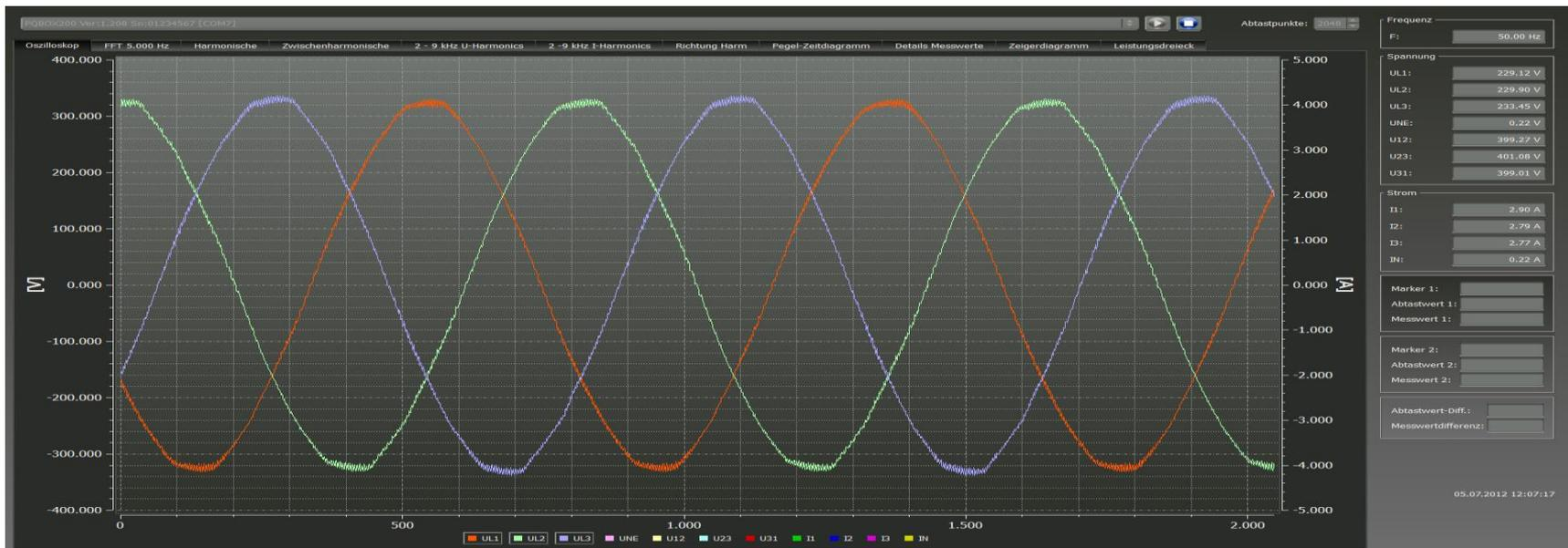
Voltage L1 / L2 / L3 at CPC (Point of Common Coupling) – caused by an Solar Inverter
