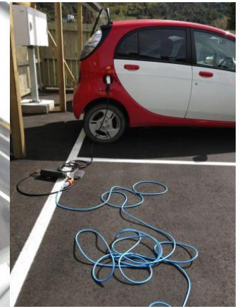
Figure 4: In-Line AC Charger
